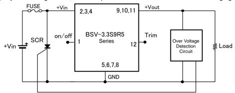
Note 1: ON/OFF control does not function in case of overvoltage mode damage.
