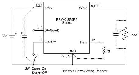
Note1: Keep ON/OFF pin open when not using ON/OFF control.
