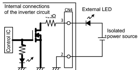
In this case the maximum current flowing through the CN4-3 pin will be 9mA. Maximum voltage that can be applied to the CN4-3 pin is 50V. When using external LED, make sure that these maximum allowable voltage and current are not exceeded.
