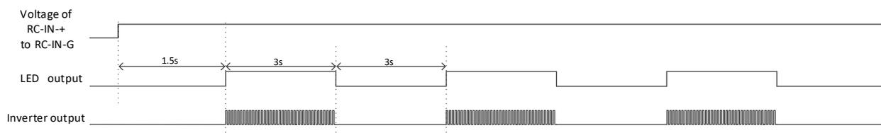
5-9-3. Protection operation: used when the power transmitting mode detects overcurrent (see chapter 5-6)
