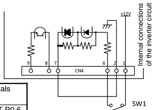
Since the internal circuit of the ON / OFF control function is electrically isolated by photo coupler, it can also be used when external circuit must be electrically isolated from the module. Electrically isolated RC signal can be used as output synchronized with ON / OFF state.
