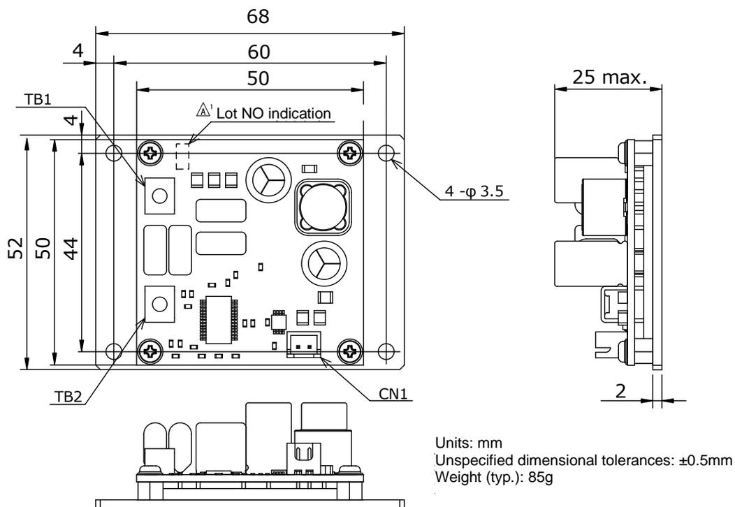
7-3-2. Appearance and dimensions of the power receiving transformer
